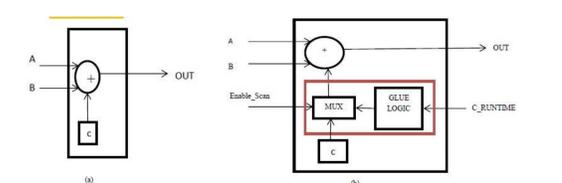
(a) Normal design example, (b) proposed scan-chain methodology for the design example in (a).
