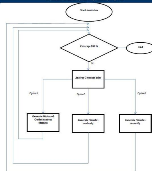
The proposed GA methodology to speedup coverage closure. Using genetic algorithms, there is no test redundancy
