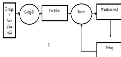
Proposed Emulation Flow (online flow), synthesizable testbench methodology, scan-chain methodology, a) detailed, b) simplified.
