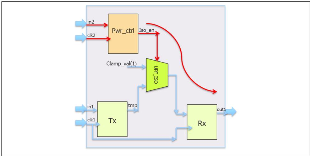
Figure 3. Isolation cell introduces a CDC path between synchronous registers
