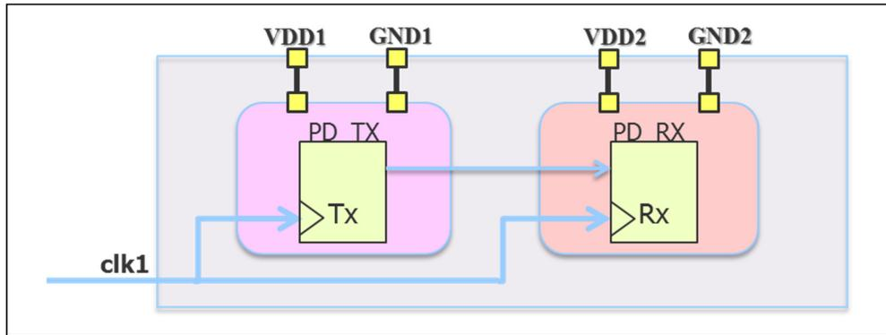
Figure 6. Synchronous registers on different voltage domains considered new CDC path
