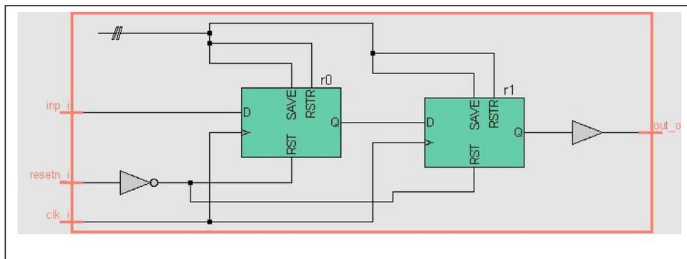
Figure 7. Retention synchronizer for VDC paths
