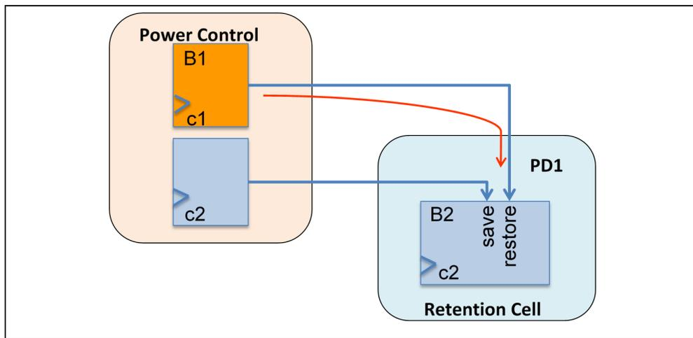
Figure 5. Retention cell introduces a CDC path to its restore pin
