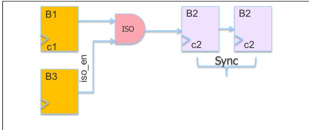
Figure 4. Isolation cell introduces a combinational logic violation
